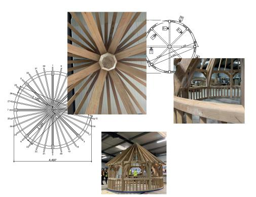
\*Price £18,525 + VAT - For the design, fabrication and supply (ex works) of all the structural oak framing including oak rafters, oak balustrading to 6 sides, padstones and associated components. The figures quoted are exclusive of VAT, taxes and import duties as applicable. Our quotation excludes shipping, groundworks, erection and roof battening/tiles.
